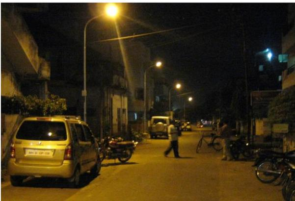
**Fig 3: Lighting Arrangement with 50 Watt Sodium Vapor Lamps**
