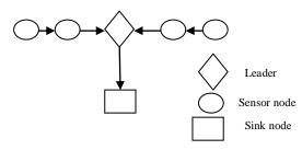
Fig 10 Chain based architecture
