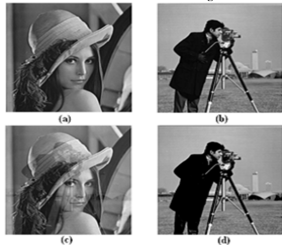
Fig. 2.2. The figure shows (a) the Lena image (b) the original Cameraman image to be watermarked (c) visible watermarked Image and (d) the recovered cameraman image.
