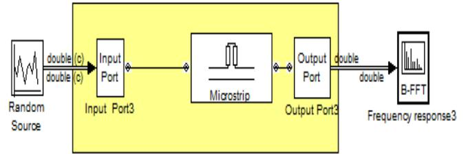
Fig.8. Modeling a Micro strip transmission line in MATLAB
