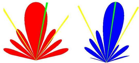
Fig. 1. Switched beam and adaptive antenna strategy for locating the target
