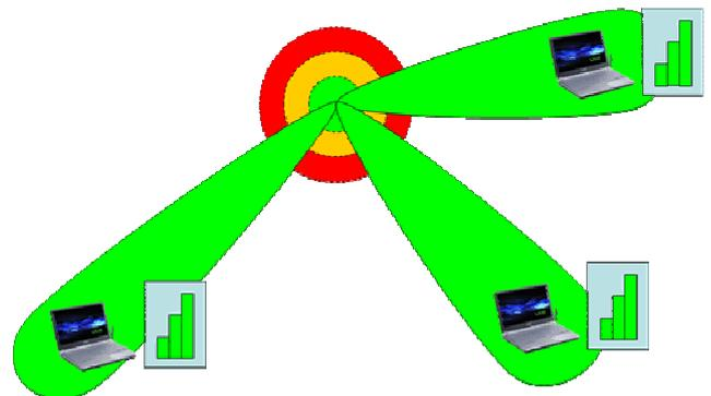
Fig.6. Adaptive Antennas technology focuses signal towards multiple users
