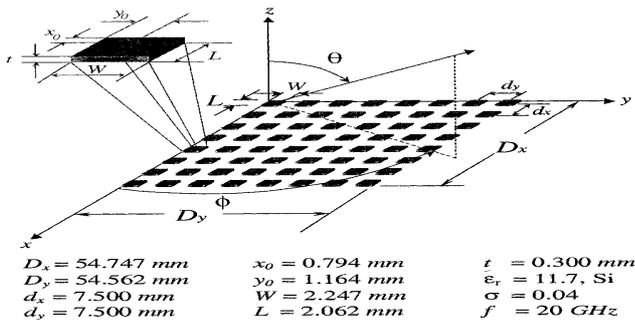
Fig. 7. A planar Array Configuration [7]
