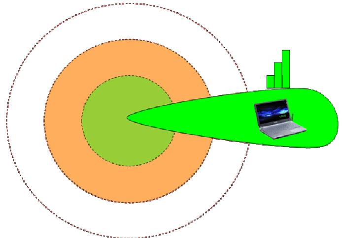
Fig. 5. Adaptive Antenna array focusing in the direction of user and hence increasing the range
