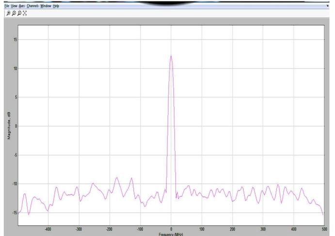
Fig. 9. Frequency Response of the Microstrip transmission line obtained at FFT scope
