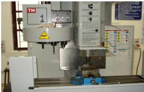
**Fig.1 Experimental set up of vertical machining center**
