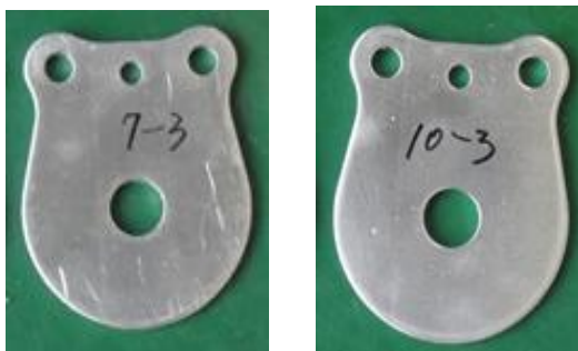
Fig. 11: General blanking product of SCM415H according to clearance
