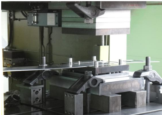
Fig. 8: Press tryout of the general blanking die
