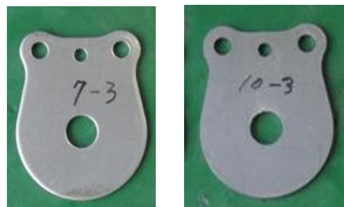
Fig. 10: Burnish surface measurement of fine blanking product
