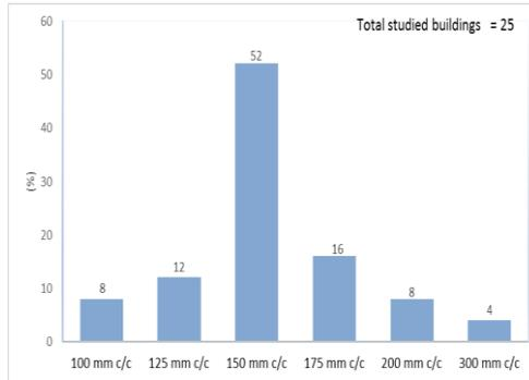
Fig 8.c : Stirrups spacing at mid of columns
