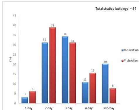
Fig 0.b: Numbers of bays in both direction
