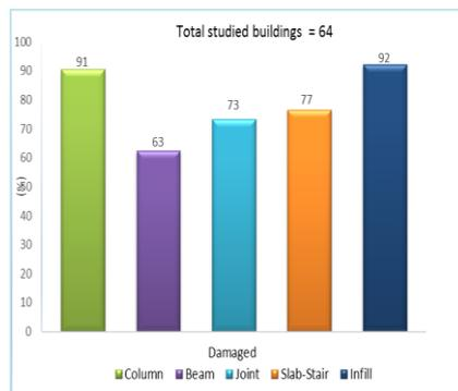
Fig 11.e : Damage of structural elements
