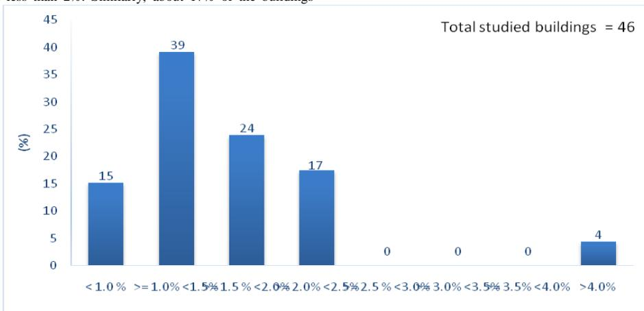
Fig 8.a : Longitudinal reinforcement percentage in columns
