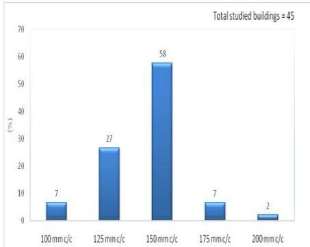
Fig 8.b : Stirrups spacing at support of columns
