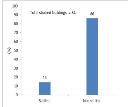
Fig 11.c : Classification of buildings according to settlement
