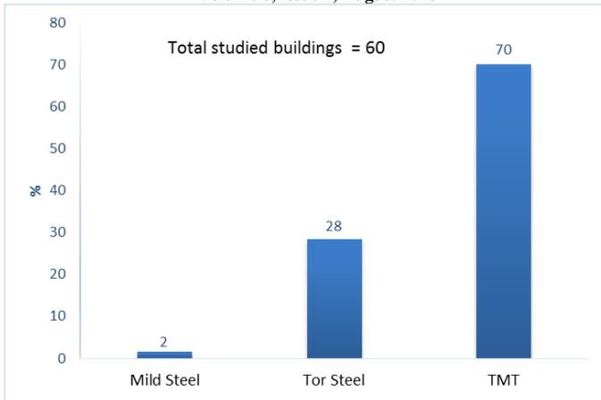
Fig 10.c : Buildings with different types of reinforcements
