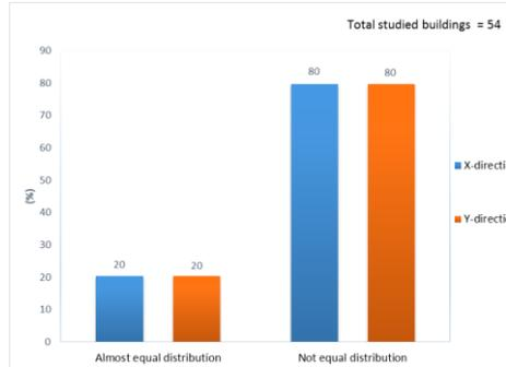
Fig 0.d : Distribution of infill walls
