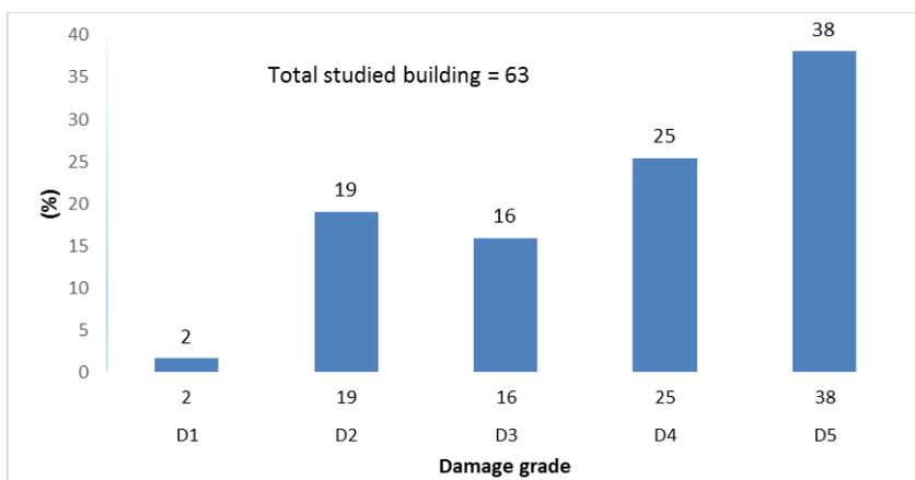
Fig 11.a : Classification of building based on damage grade
