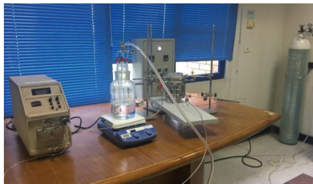
Fig. 3 Flow setup of the cooling system
