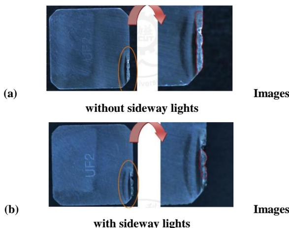
Fig. 8 Images without and with sideway light sources
