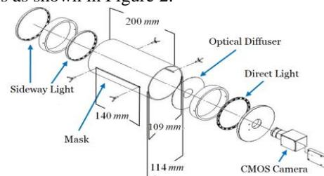
Fig. 1: The structure of the designed photo mask.
