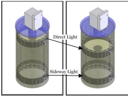
Fig. 2: Adjustment of light positions by the screws.
