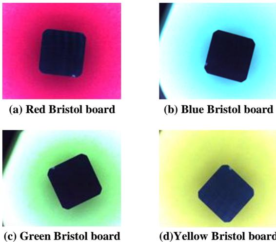
Fig. 3: Using Bristol boards as backgrounds.
