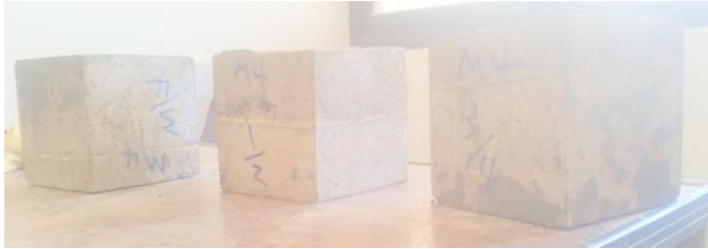
Fig (2) Cubes Samples with FCJ at quarter, middle and three quarters
