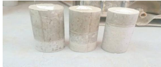
Fig (4) Cylinders Samples with FCJ at quarter, middle and three quarters
