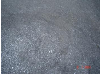
Plate 1: Steel slag used as fine aggregate [5]
