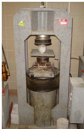
Plate 4: Splitting tensile Test conducted on concrete specimen [2]
