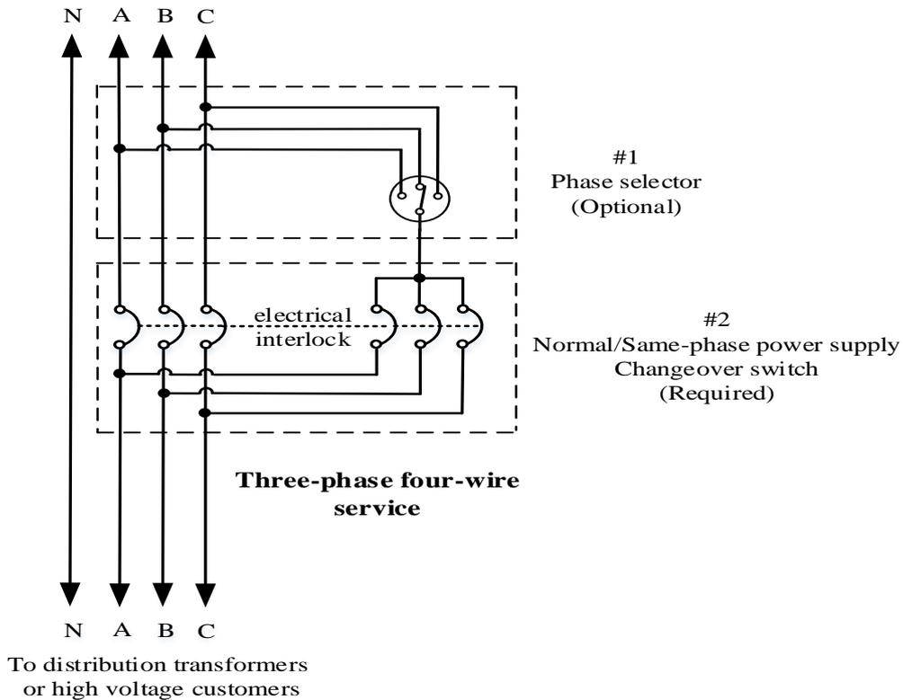
Fig. 2: Circuit for applying the SPPS scheme in a 3φ4W service
