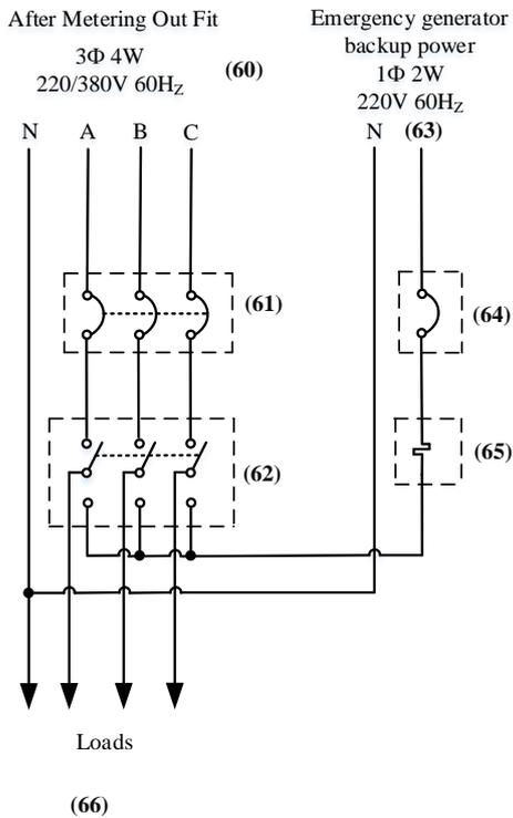
Fig. 5: Circuit with manual operation function designed for 3 $\Phi$ 4W services
