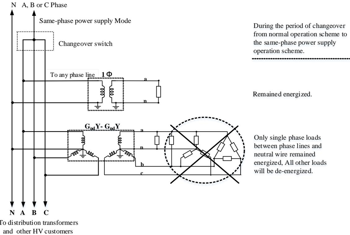
Fig. 1: Applicable wiring and load connections to apply the SPPS scheme
