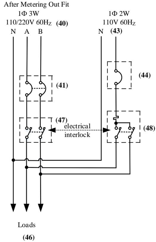
Fig. 4: Circuit with automatic operation function designed for 1 $\Phi$ 3W services
