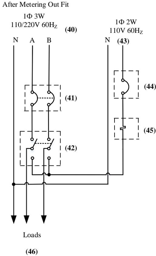
Fig. 3: Circuit with manual operation function designed for 1 $\Phi$ 3W services
