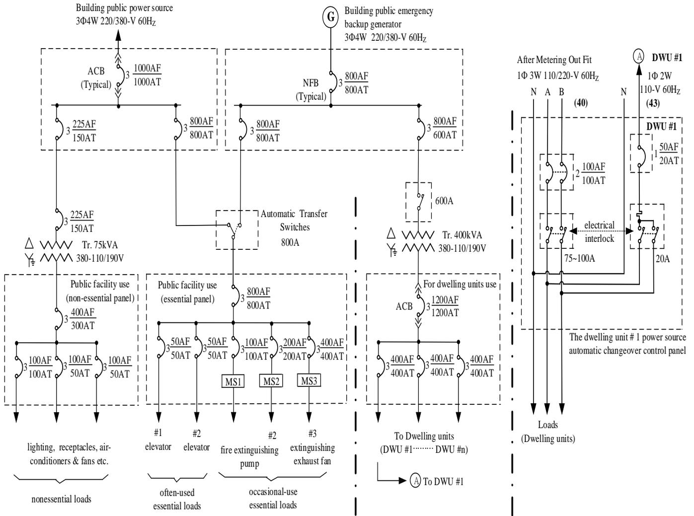
Fig. 7: Single-line diagram of application of the SPSS scheme during an emergency power supply period
