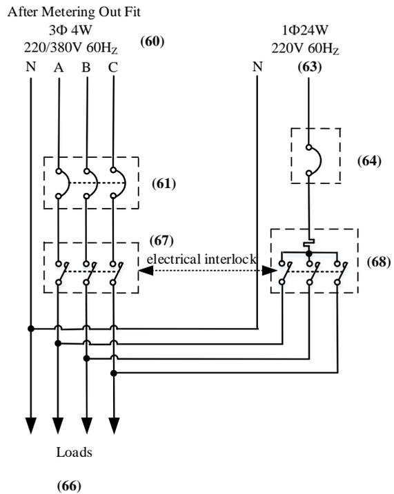
Fig. 6: Circuit with automatic operation function designed for 3 $\Phi$ 4W services
