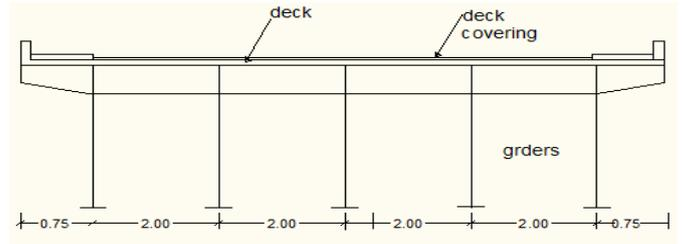
Fig.5a : Cross Section of the Bridge
