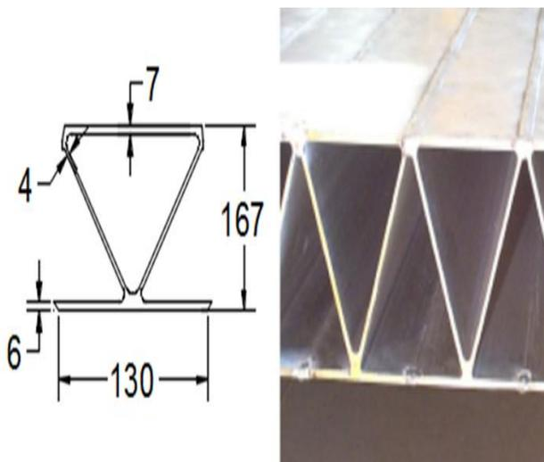
a- Cross-Section of the Aluminum Deck Panel,
