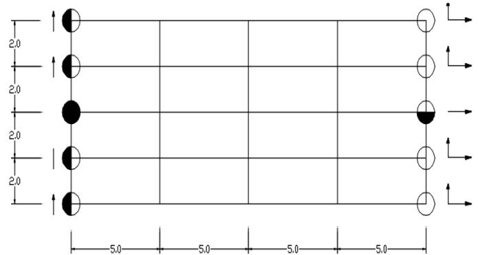
Fig.5b: Plan of the Bridge Dimensions in m
