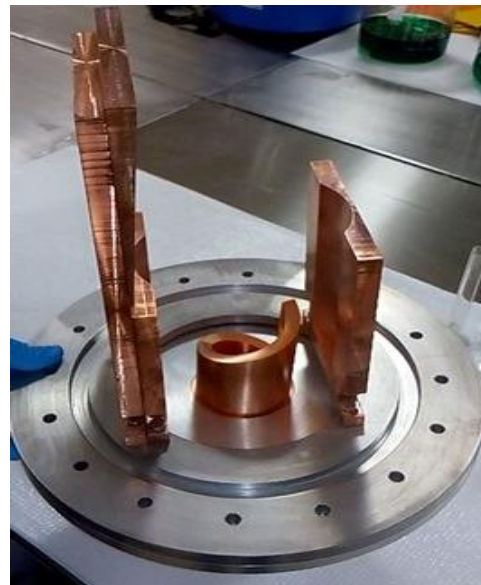
Fig.7 Quasi optical mirrors system of Gyrotron
