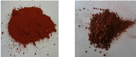
Fig. 1. Fe 2 O 3 nanoparticles before and after sintering
