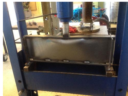
Fig 10. Beam with no internal stiffeners, Configuration I, after web buckling
