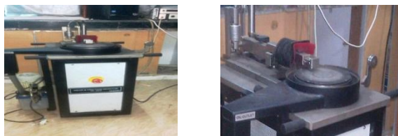
Fig: 3, Machine for conducting wear test (pin on disc wear testing machine)
