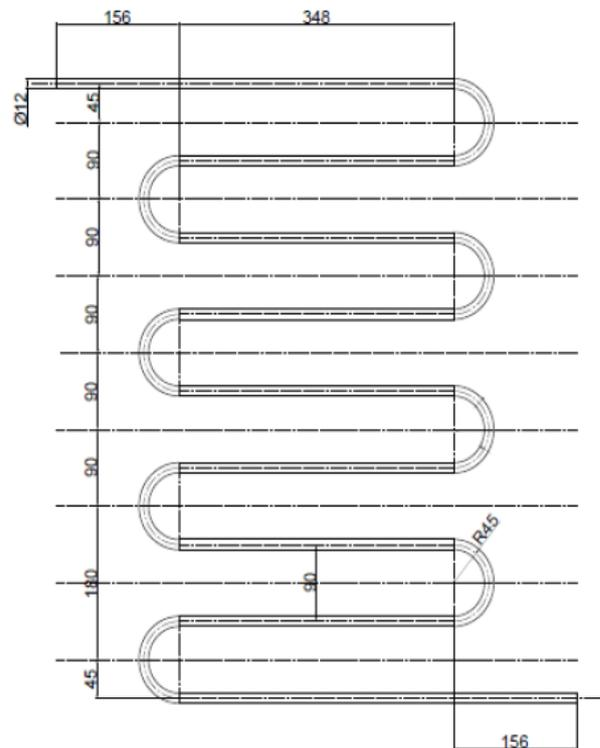
Fig 5 A detailed drawing for copper tubing of the designed solar flat plate collector
