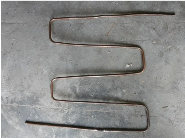
Fig 7 A photographic view of the Serpentine copper tubing of the designed solar flat plate collector
