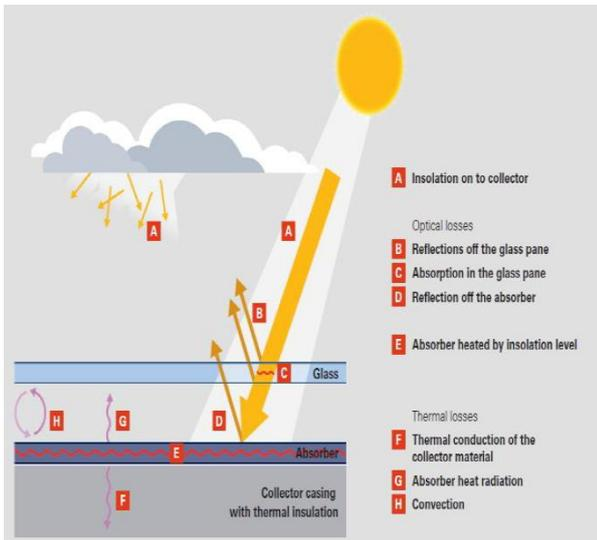
Fig.8 Energy flow in the collector
