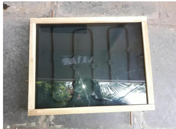
Fig.1 Flat plate collector used in the experiment
