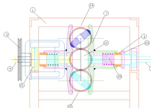
Fig.1. CAD Model of Half Toroidal CVT
