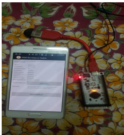
Fig.10 LED On when it is interfaced with Bluetooth device
