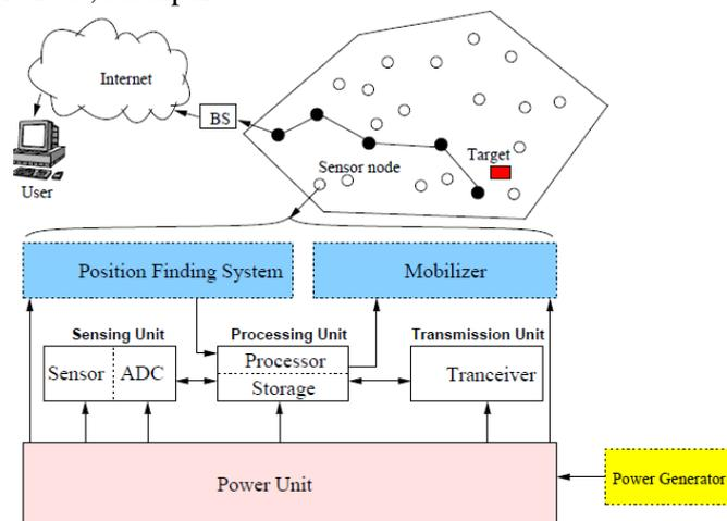
Fig 1: sensor node component and Network [3]
