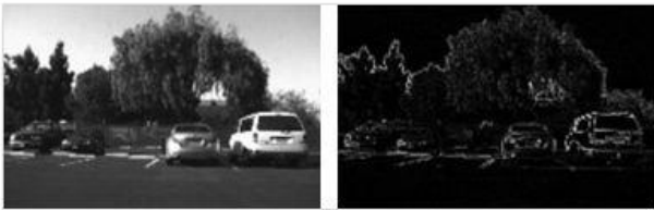
Fig.1 Image segmentation using Sobel method [32]
