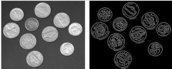
Fig.2 Image segmentation using Canny method [32]
