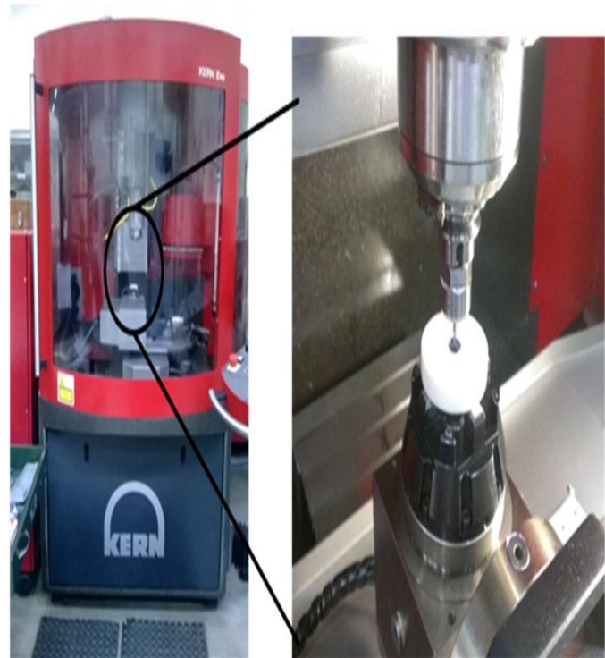
Fig.4. a) Teflon mold on which microneedle holes are made, b) Microholes drilling on micromachining centre
