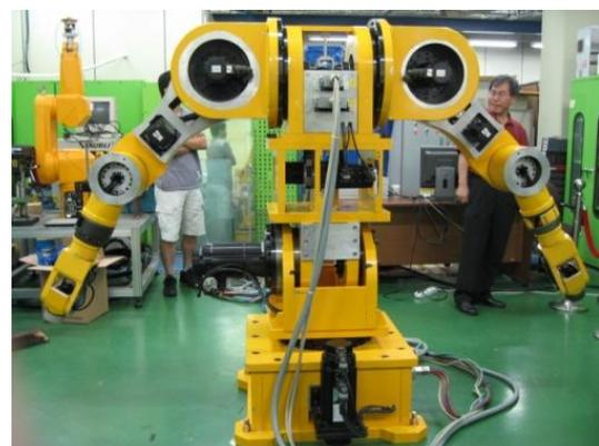
Fig. 4 Developed dual arm robot manipulator
