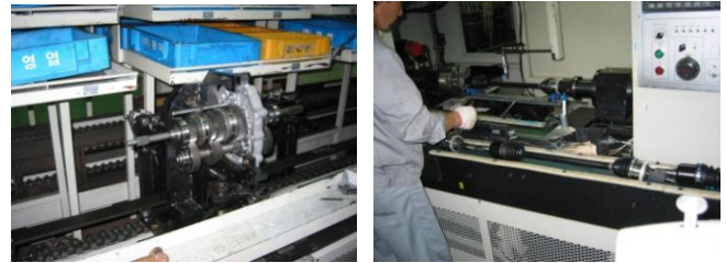
Fig.1 Transmission assembly line (left) and the CV Joint assembly line
