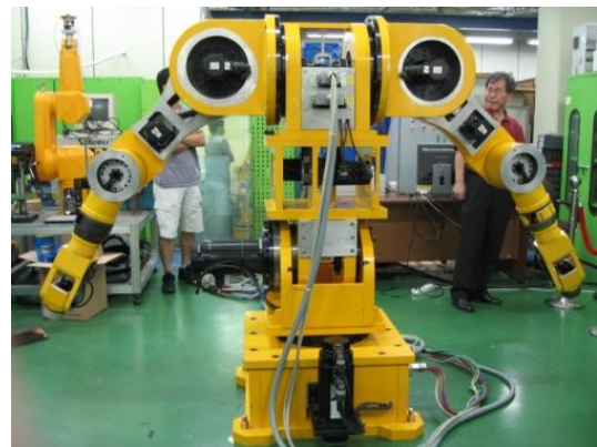
Fig. 4 Developed dual arm robot manipulator
