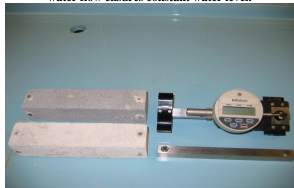
Fig 2. Test apparatus and specimens with DEMEC points attached to the surface used for the evaluation of Moisture Movement.
