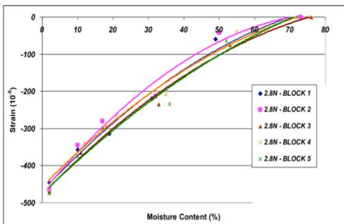
Fig 4. Graph of Moisture Movement for 2.8N Aircrete using DEMEC Points.
