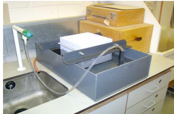
Fig 1. Test set-up for water absorption test. The block is immersed in water to a depth of 5 mm ± 1mm. Continuous water flow ensures constant water level.
