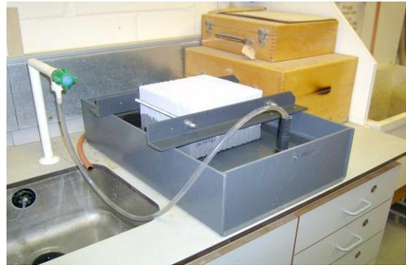
Fig 1. Test set-up for water absorption test. The block is immersed in water to a depth of 5 mm ± 1mm. Continuous water flow ensures constant water level.
