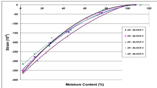
Fig 3. Graph of Moisture Movement for 2N Aircrete using DEMEC Points.
