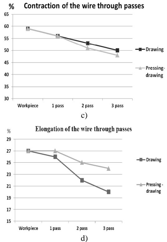
**Fig. 4 - Graphs of depending mechanical properties of the copper samples from number of passes**
