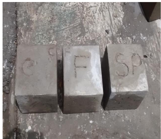
Fig.2 Sulphate attack on cubes
