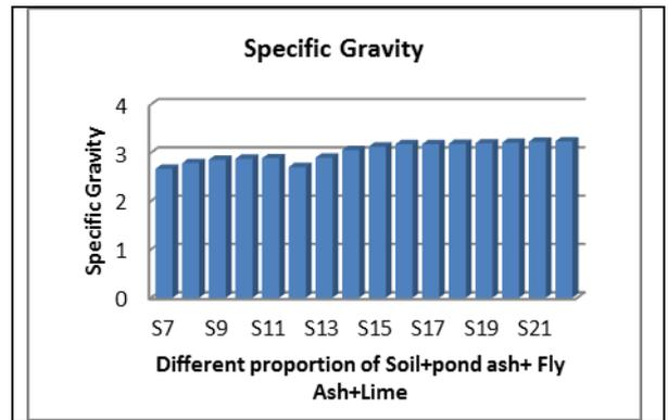
Fig 4; Result of Specific Gravity
