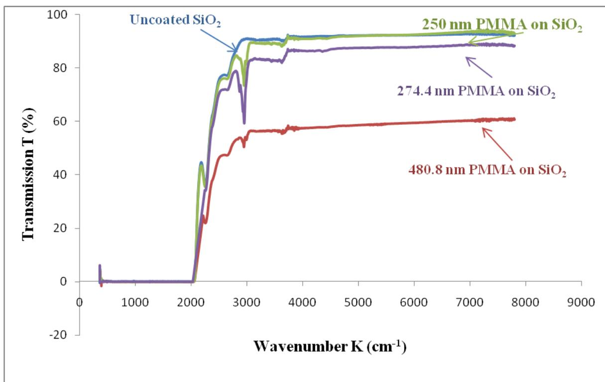
Fig. 2: FTIR spectra comparing the infrared transmissions through SiO<sub>2</sub> coated with PMMA film layers of different thickness.
