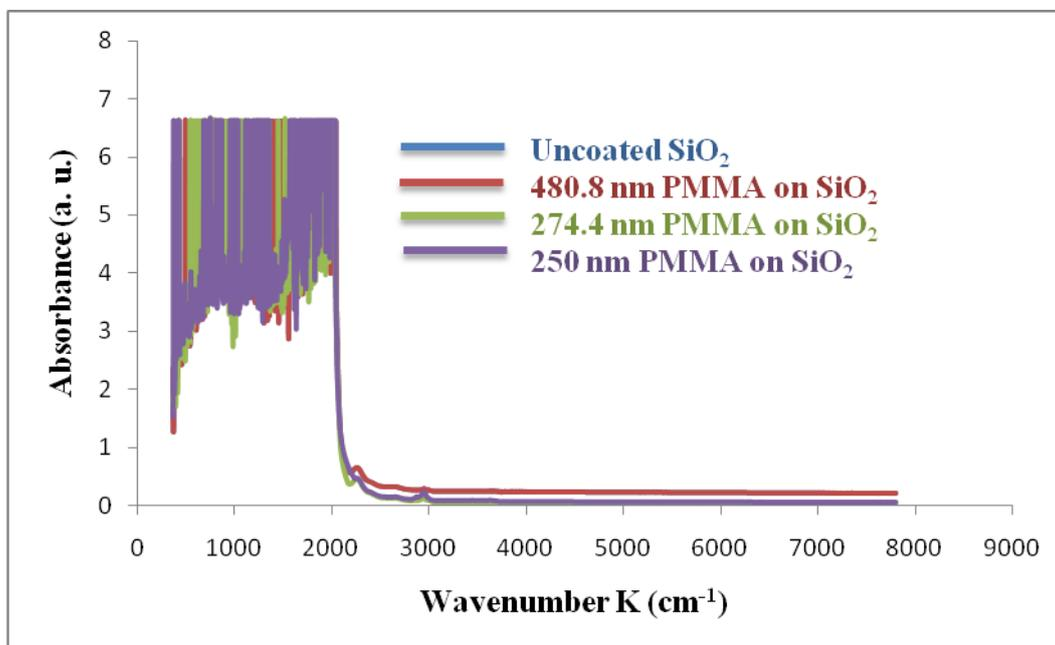
Fig. 3: FTIR spectra comparing the infrared absorptions on SiO<sub>2</sub> coated with PMMA film layers of different thicknesses.
