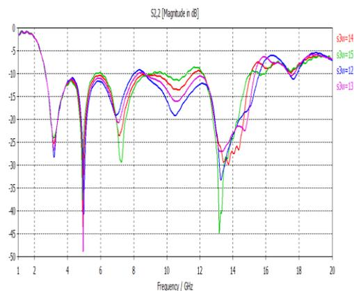
**Fig 5: S- parameter graph on different slot length**
