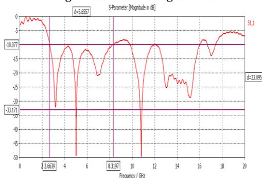
Fig 8: The s- parameter graph of feedline edge cut antenna
