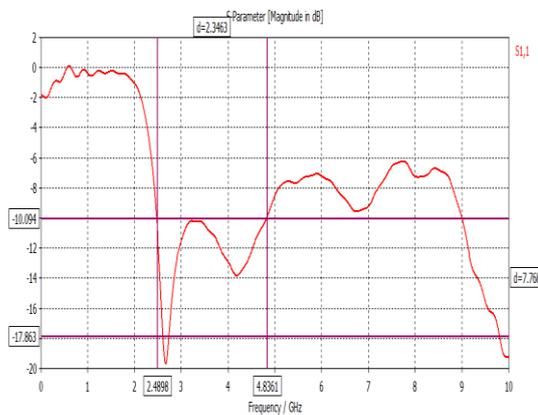
Fig 10: S parameter graph of a slot antenna backed by a metal box
