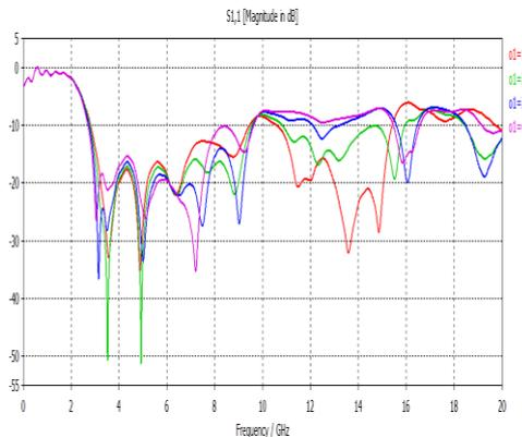
**Fig 4:: S-parameter graph showing different feed position effects**
