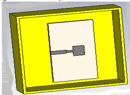
Fig 9: Slot antenna backed by a metal box
