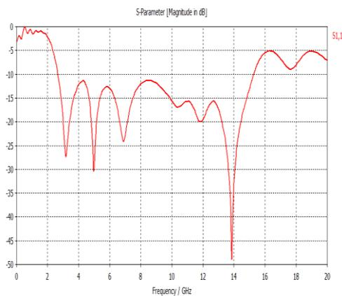
**Fig 3: Simulated S-parameter of the antenna**
