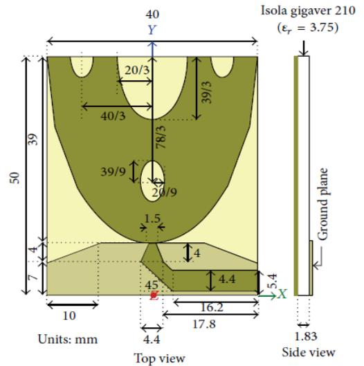
Fig. 3: The configuration of UWB antenna as in [9].
