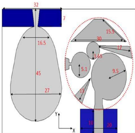
Fig. 15: Rotatable reconfigurable multi-antenna [7].
