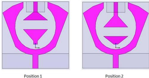
Fig. 14: The cognitive antenna structure.
