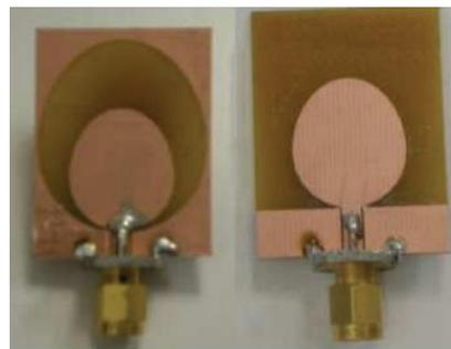
Fig. 5: UWB antennas with optimized ground planes [10].
