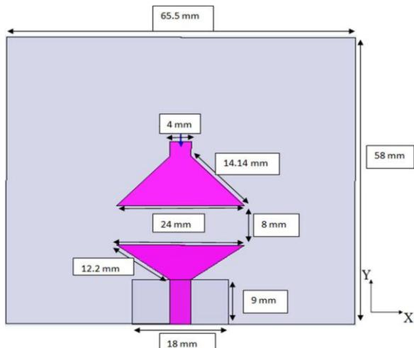
Fig. 10: The “reconfigurable communicating” antenna structure.
