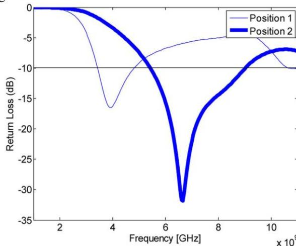
Fig. 12: Return loss of reconfigurable communicating antenna.
