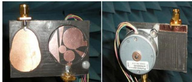
Fig. 16: Fabricated prototype of Fig. 15 [7].
