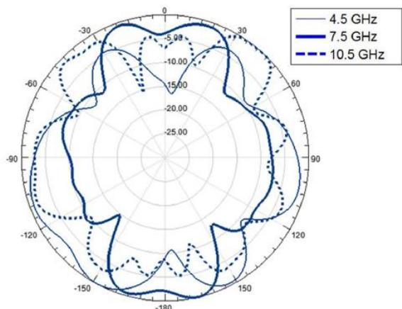
Fig. 9: The normalized radiation pattern of sensing antenna.
