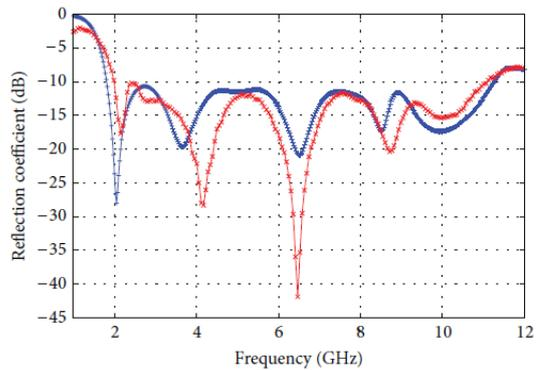
Fig. 4: Reflection Coefficient of the UWB antenna in Fig. 3.
