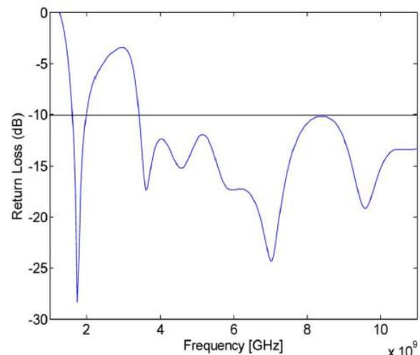
Fig. 8: Return Loss of Sensing antenna.
