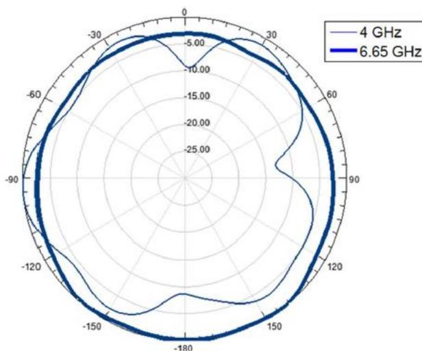
Fig. 13: The normalized radiation pattern for positions 1 and 2.
