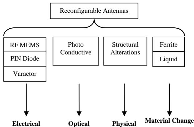
Fig. 6: Implementation of Reconfigurable Antennas [3].
