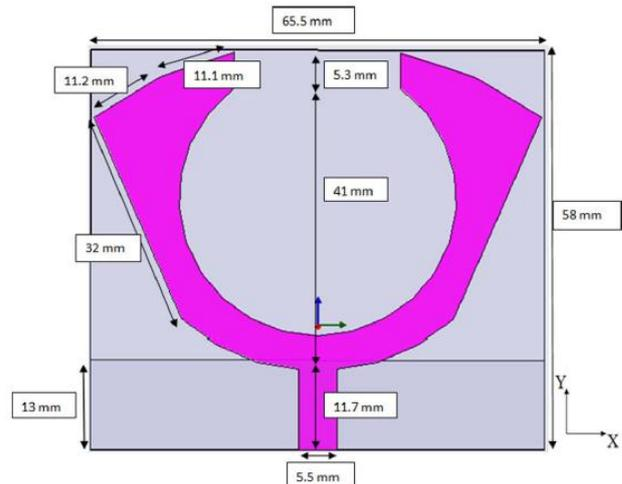
Fig. 7: Sensing antenna
