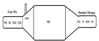
Fig .1 Working of the system in exhaust manifold
