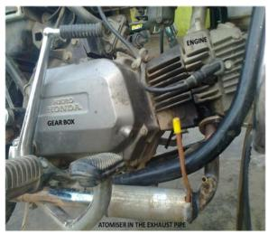
Fig 2 Atomizer in the exhaust manifold
