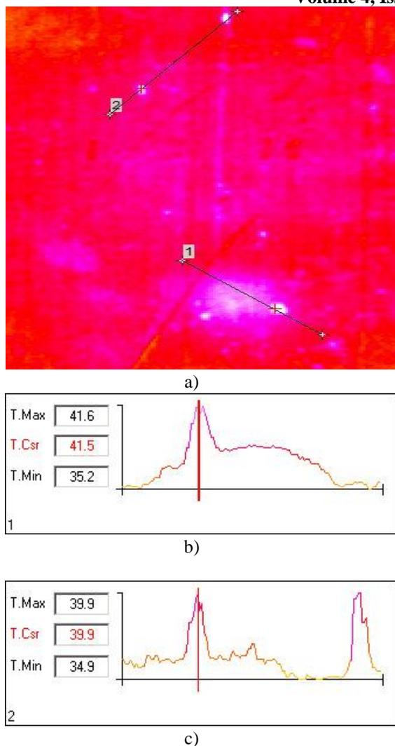
**Fig. 1. The thermo gram surface temperature of the mixture (a). The graphs of temperature change along the sections 1, 2 (b, c). Beginning of the manufacturing process.**
