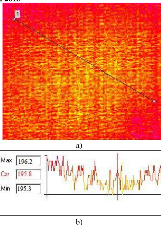
**Fig. 2. Thermo gram of temperatures on surface of the mixture (a). Graph of change of temperatures on surface of the mixture (b). Melting polystyrene.**
