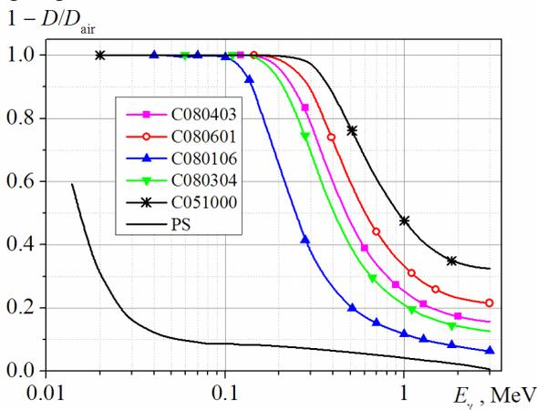
**Fig. 4. The weakening of the absorbed dose of gamma radiation with a protective layer of the composite material of the second group.**
