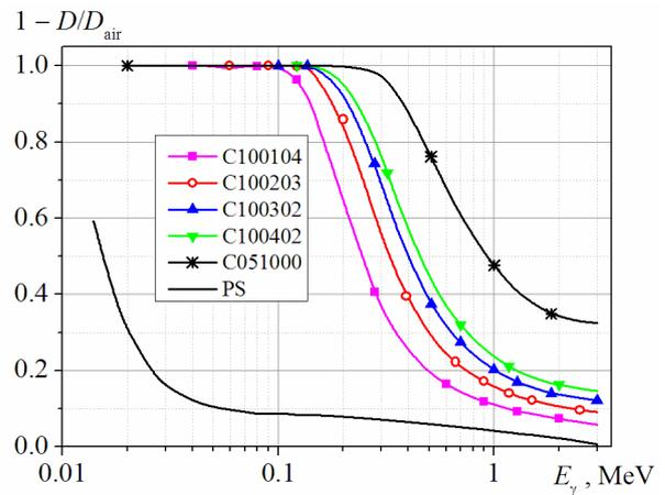
**Fig. 5. The weakening of the absorbed dose of gamma radiation with a protective layer of the composite material of the third group.**
