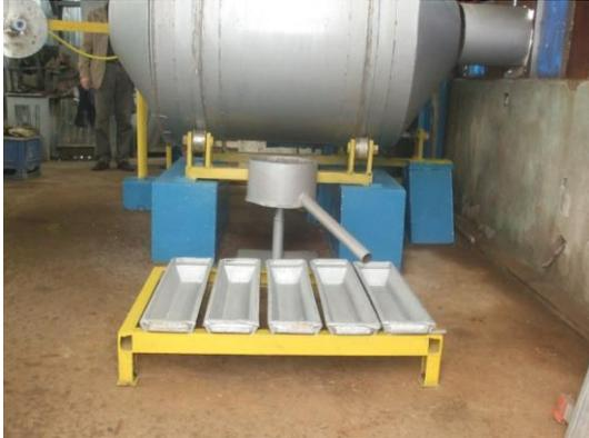
Fig. 2. System used for casting phase lead into ingot molds
