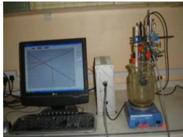
Fig (2): the electrochemical corrosion unit.
