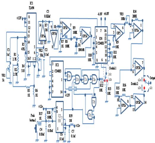
**Fig. 1. The detail schematic of one shot bipolar saw tooth-like waveform converter.**
