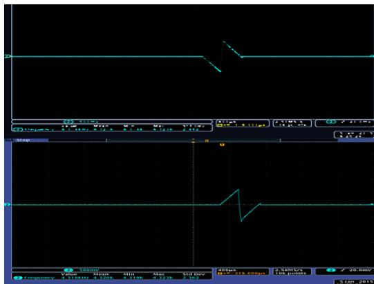
**Fig 2 the upper trace represents the backward direction and the lower trace indicates the forward direction for a stick-slip motion PZT driver**
