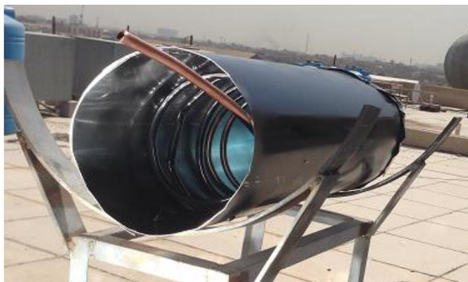
Fig (3), Experimental cylindrical receiver.
