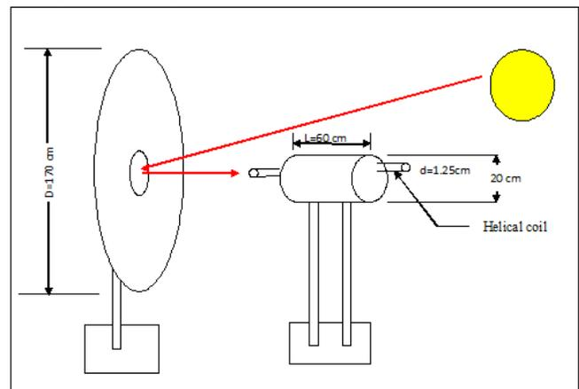
Fig (1) schematic diagram of concentrated solar dish.
