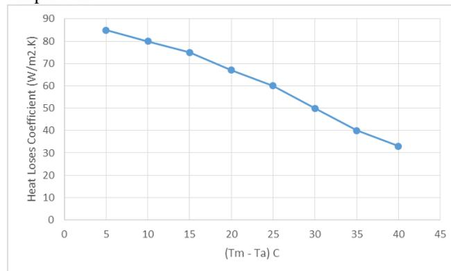
Fig (6) variation of heat loss coefficient by radiation with operating temperature of receiver.
