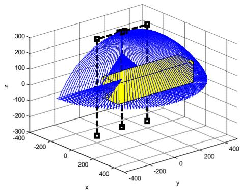
Fig. 3 Workspace analysis of dual arm robot (Length parameter 200mm, 400mm)
