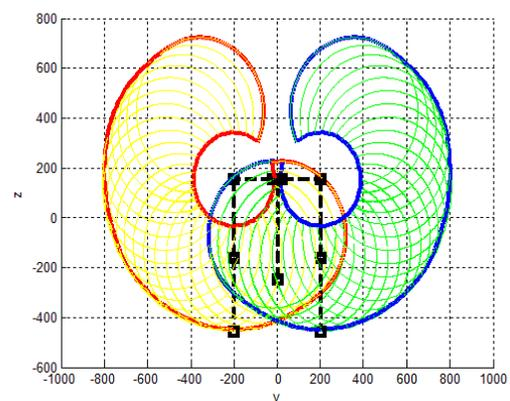
Fig. 2 Workspace analysis of dual arm robot
