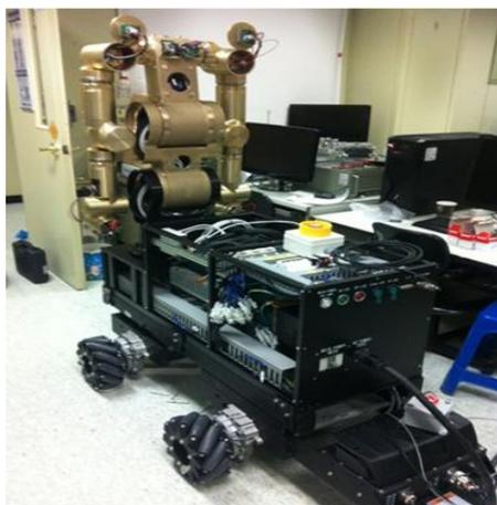
**Fig. 8 Dual arm robot with the mobile platform**
