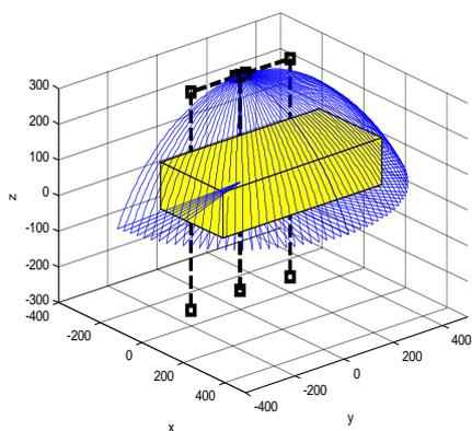
Fig. 4 Workspace analysis of dual arm robot (Length parameter 300mm, 300mm)
