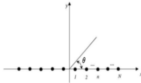
**Fig 1. Geometry of the  $2N$  element linear antenna array with uniform spacing**
