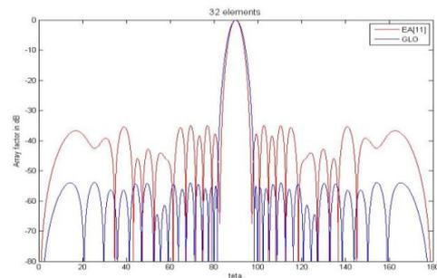
Fig 5. Array factor for 32 elements
