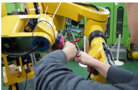
Fig 9 Direct teaching of a dual arm robot manipulator using the developed easy teaching interface
