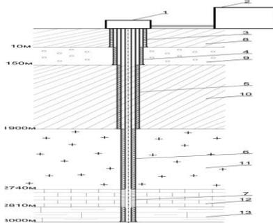
Fig.4. The scheme of wastewater disposal into deep horizons
