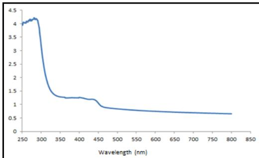
**Fig (1) the absorption spectrum of CdS**
