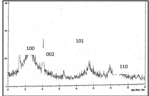
**Fig (4) XRD for CdS nanoparticles**
