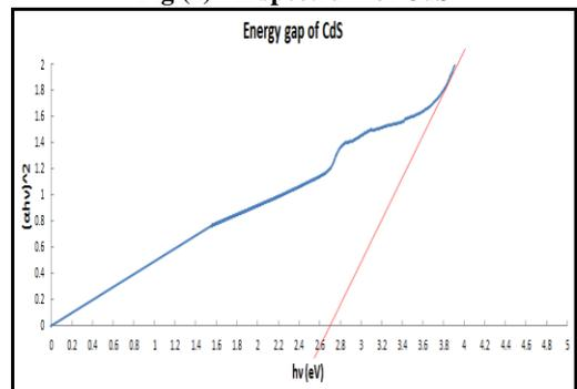
**Fig (3) The band gap of CdS**
