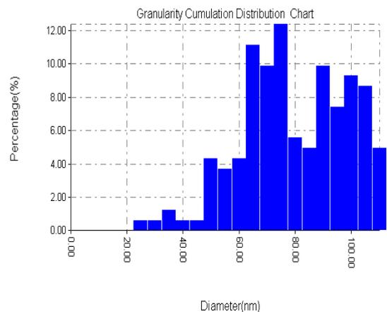
**Fig (5) AFM Measurement for CDS Nanoparticles**
