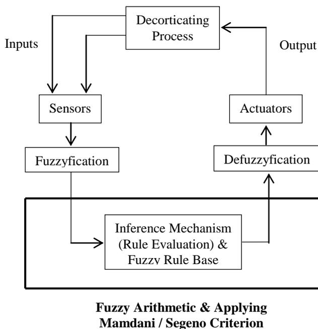
Fig. 1: Decorticator Fuzzy Logic Controller (D-FLC) [[2]-[5]]
