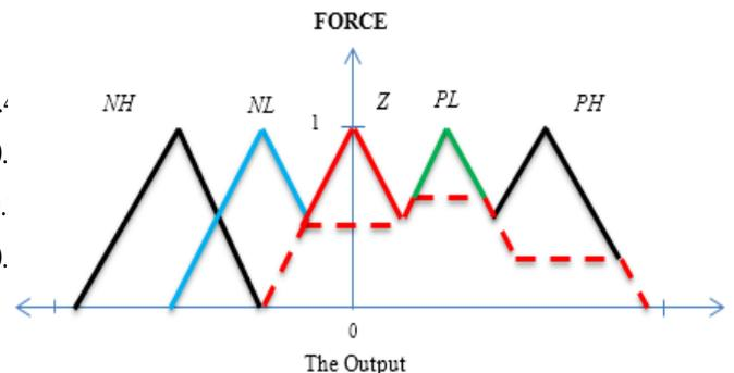
Fig. 5. The fuzzy set of the output force
