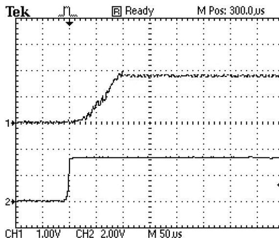
**Fig. 7 Measured waveform of  $v_{out}(t)$  at the power-up transient**
