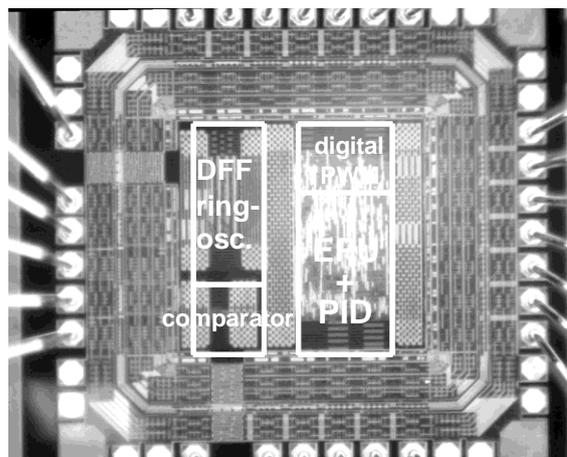
**Fig. 6 Chip microphotograph of the proposed PWM controller IC**
