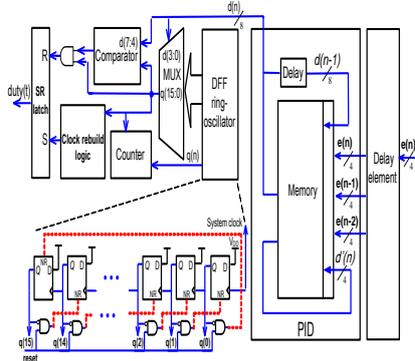
**Fig. 4 Block diagram of the multiple-access PID compensator and digital PWM**
