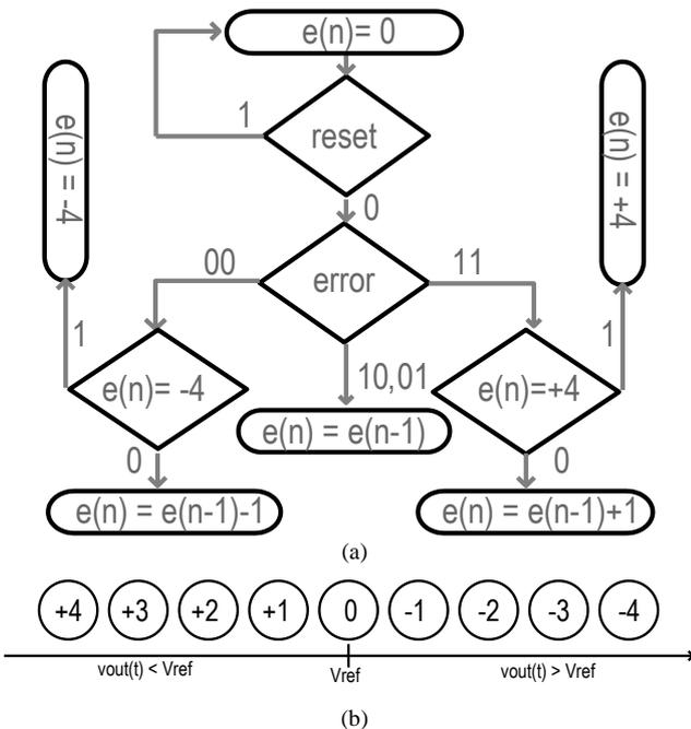
**Fig.3 (a) Operation diagram of the 4-level EPU (b) State relationships with the two compared voltages**
