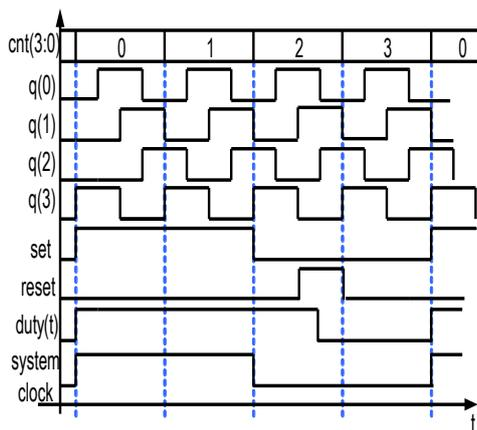
**Fig. 5 Operation timing of a simplified 4-bit digital PWM**
