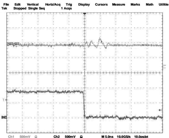
Fig. 9 Waveforms for line transient response ( $V_g$  is from 4.2V to 3.3V)
