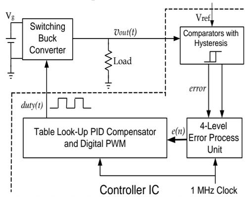
**Fig.1 Block diagram of the proposed controller for power regulation**
