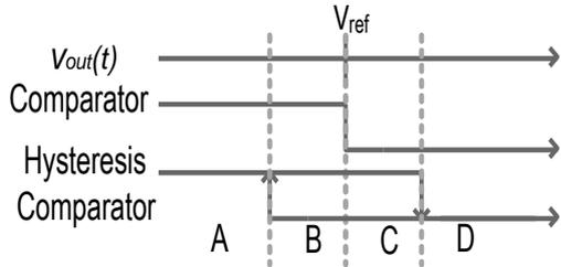
**Fig.2 Generation of the 4 levels from the comparators**
