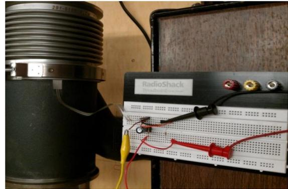
**Fig 2. Piezoelectric sensor test platform with charge mode amplifier setup**
