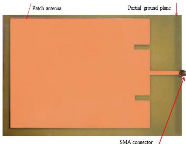
Fig. 4: Picture of fabricated wide band slotted patch antenna
