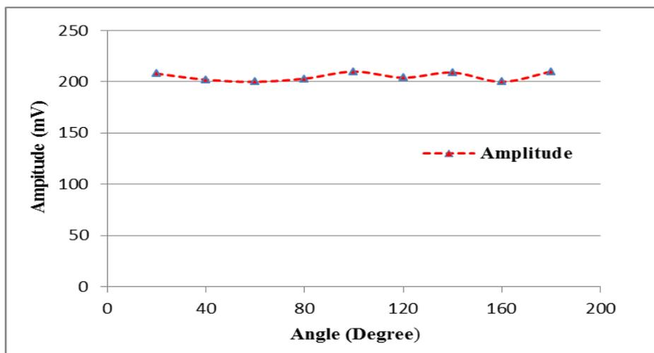
Fig. 9: Results of Radiation pattern: Amplitude versus angle (Degree)
