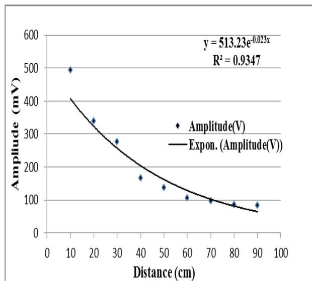
Fig. 7: Results of transient response: Amplitude verses Distance
