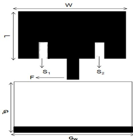
**Fig. 1: Basic configuration of wide band slotted patch antenna with feed line and partial ground plane.**
