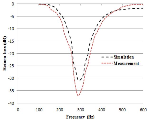
Fig. 5: Simulated and Measured results of return loss (dB) against frequency (MHz)
