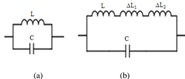
**Fig. 2: The wide band mechanism of slotted Patch antenna (a) Equivalent circuit of micro strip patch antenna (b) Equivalent circuit of E-shaped patch antenna.**
