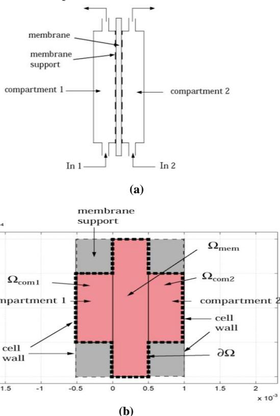
Fig 1. (a) Cell unit. (b) Boundary of separation system
