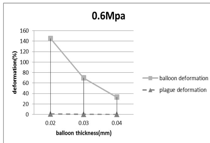
Fig. 19 Results from 0.6MPa pressure
