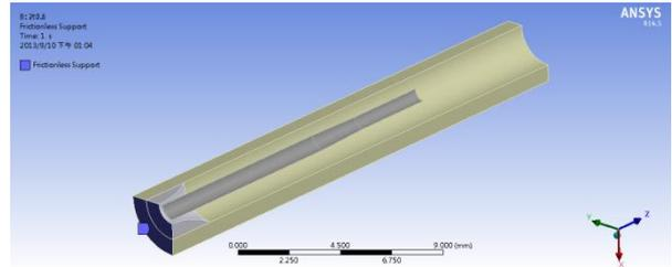
Fig. 9 Intermediate vessels joined frictionless support
