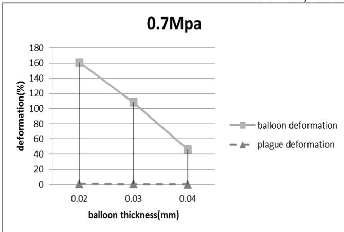
Fig. 20 Results from 0.7MPa pressure
