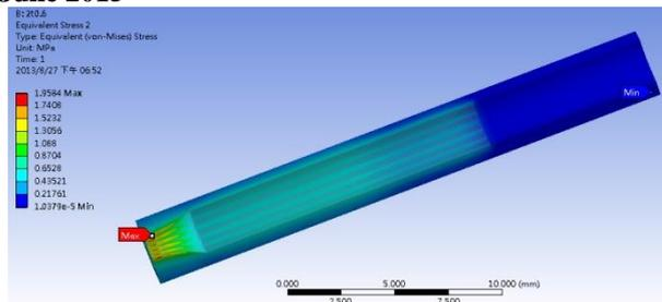
Fig. 18 Stress in plaque and vascular
