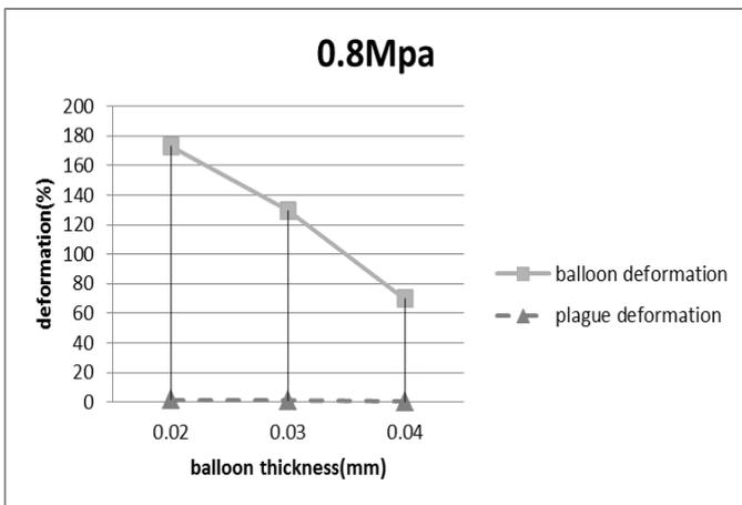
Fig. 21 Results from 0.8MPa pressure
