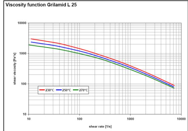
**Fig. 3 Shear viscosity curves for Grilamid L25**
