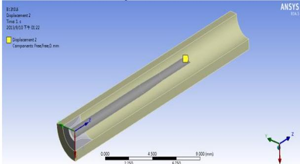
Fig. 13 The balloon cannot elongate or shorten, the balloon end of the Z-direction displacement is 0
