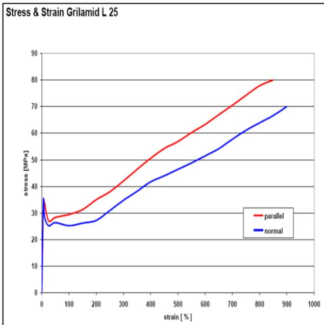
**Fig. 2 Stress-strain curve of Grilamid L25**
