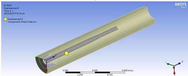
Fig. 15 Not to limit the torsional deformation of the balloon, balloon displacement in direction Y side is 0
