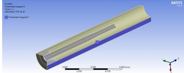
Fig. 11 Vascular underside added frictionless support
