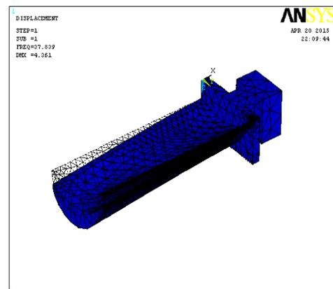
**Fig 13: Mode Shape of Turbine**
