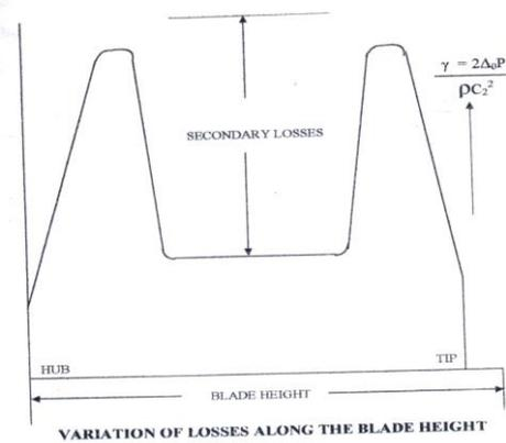
Fig.2: Loss along the Blade Height
