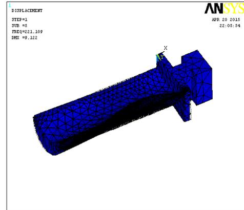
**Fig 12: Mode Shape of Turbine**
