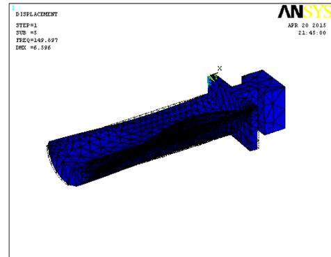
**Fig 14: Mode Shape of Turbine**
