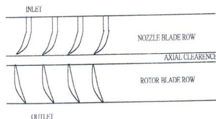
**Fig.1: A Turbine Stage**
