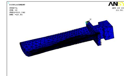
**Fig 15: Mode Shape of Turbine**
