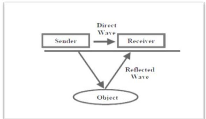
Fig 1: Illustration of different paths of reflection of radar waves
