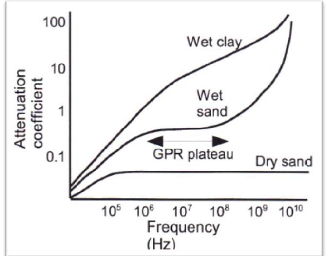
Fig.4: Illustrates the attenuation coefficient of the radar wave as a function to the frequency into the wet and dry media [Bernth Johansson, 2005; Kun Fa Leeabc, 2009].
