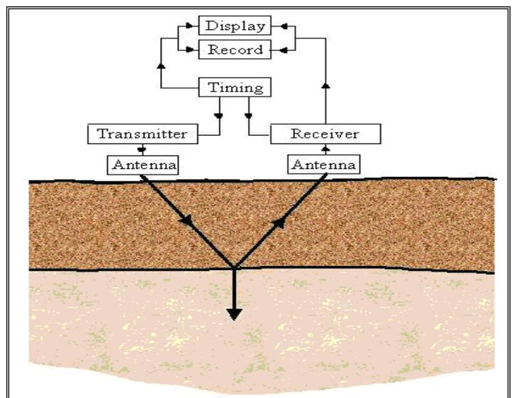
Fig 2: Illustration of the behavior of the radar waves from the beginning of transmission until it is received by receiver antenna. [Basson, 2000].
