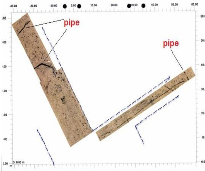
Fig 11: survey MIRA MALÅ in depth 0.63 m
