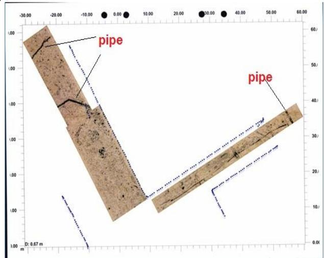
Fig 10 : survey MIRA MALÅ in depth 0.67 m
