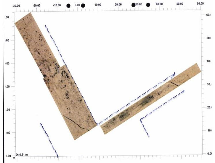
Fig 8: survey MIRA MALÅ in depth 0.51 m
