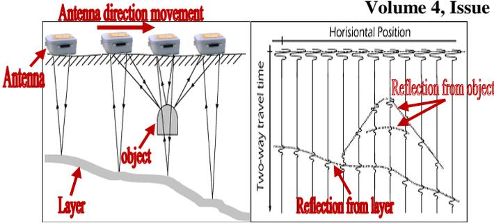
Fig 3 illustrates the principle of ground penetrating radar detection. It shows clearly that the radar wave is reflected by the buried object (on the left). The results recording are show on the right. [Hannu Luodes, 2008].
